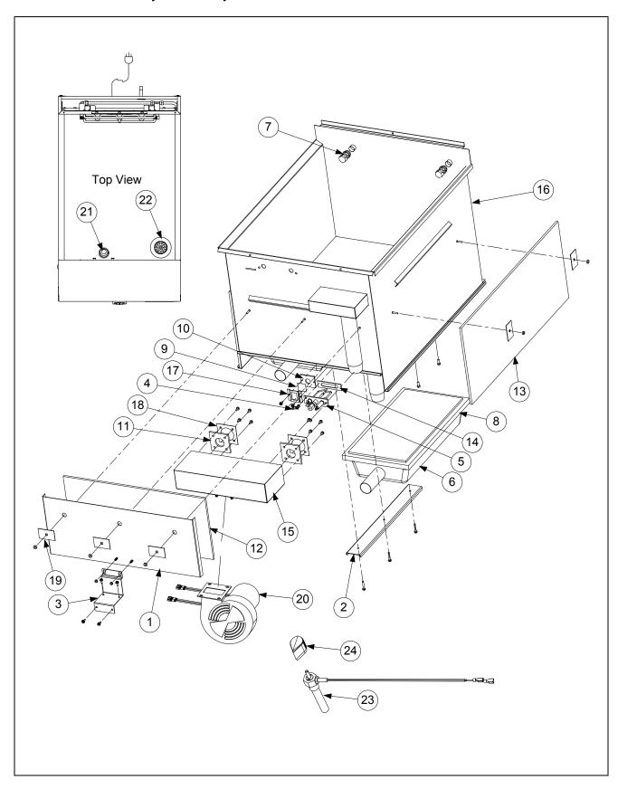
1.3 Combustion System Components cont.
